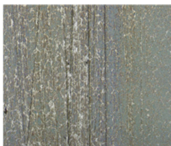
Fig. 10 (a-e): Surface condition of the small eye bearing surface before and after the tribotest.
