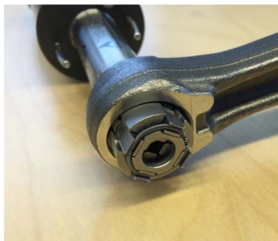
Fig. 1 Triboconditioning tool used for the treatment of small eye bearing surface.
