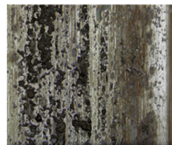
Fig. 10 (a-e): Surface condition of the small eye bearing surface before and after the tribotest.
